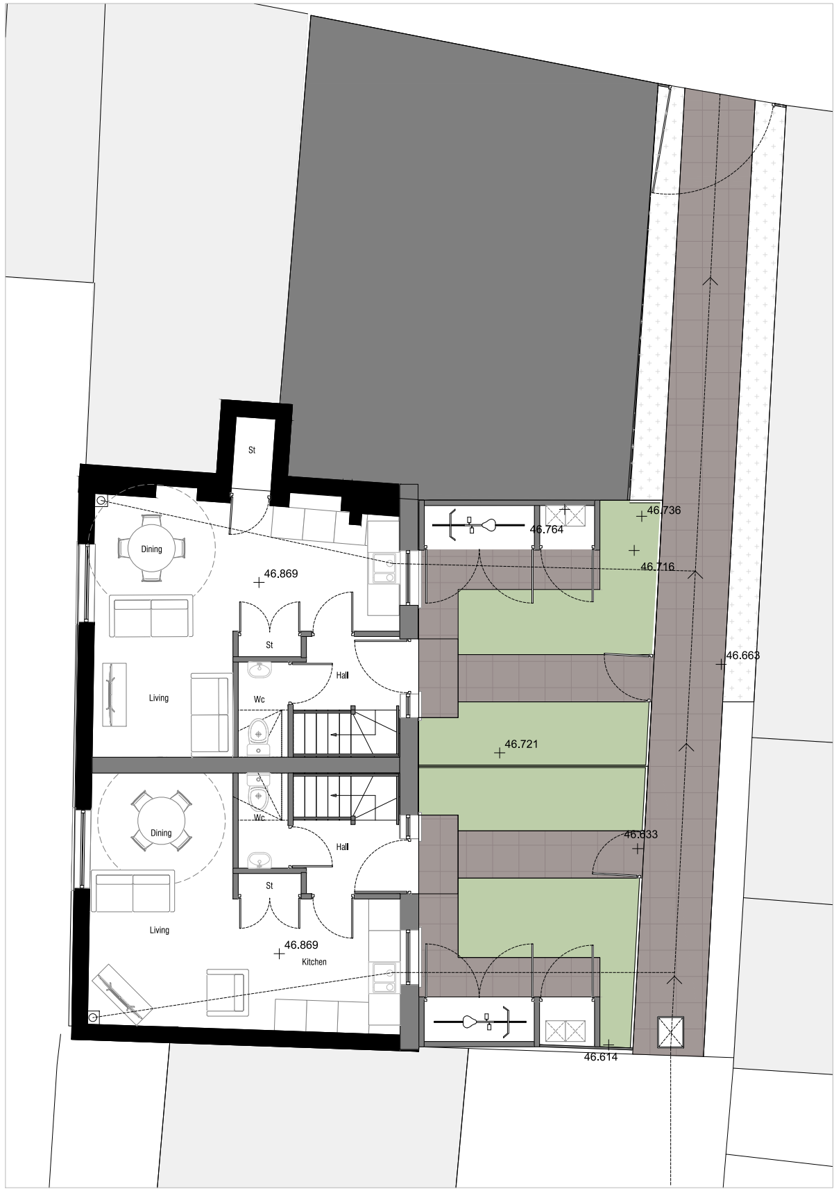
01 - Proposed Ground Floor Plan
