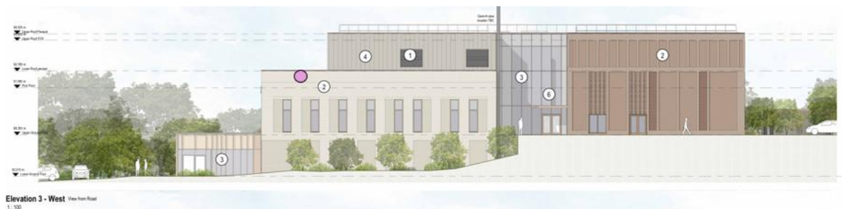
Figure 5. West elevation showing indicative positioning of three swift bricks grouped together (purple).
