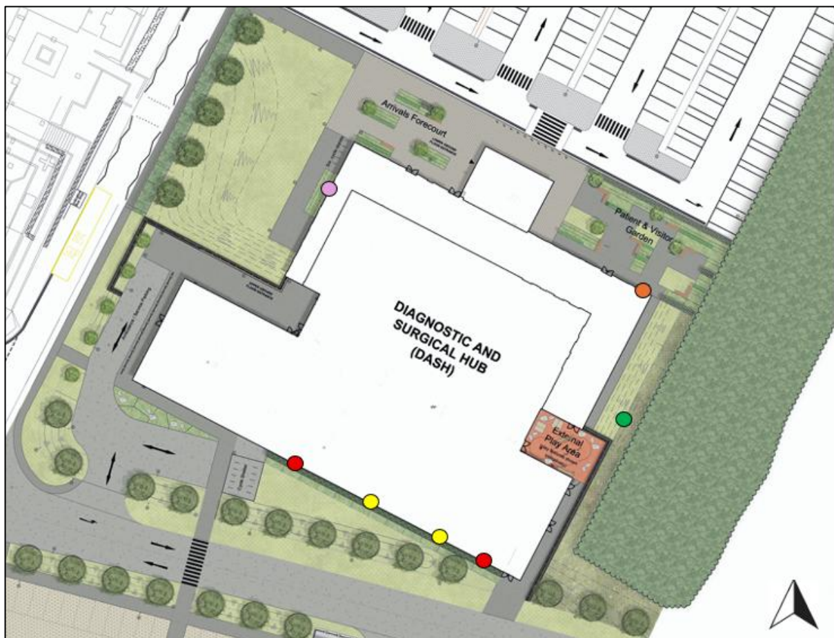
Figure 1. Location of ecological features: bat boxes (red), sparrow nest terrace (orange), swift nest bricks (purple), insect bricks (yellow) and standing log pile (green).
