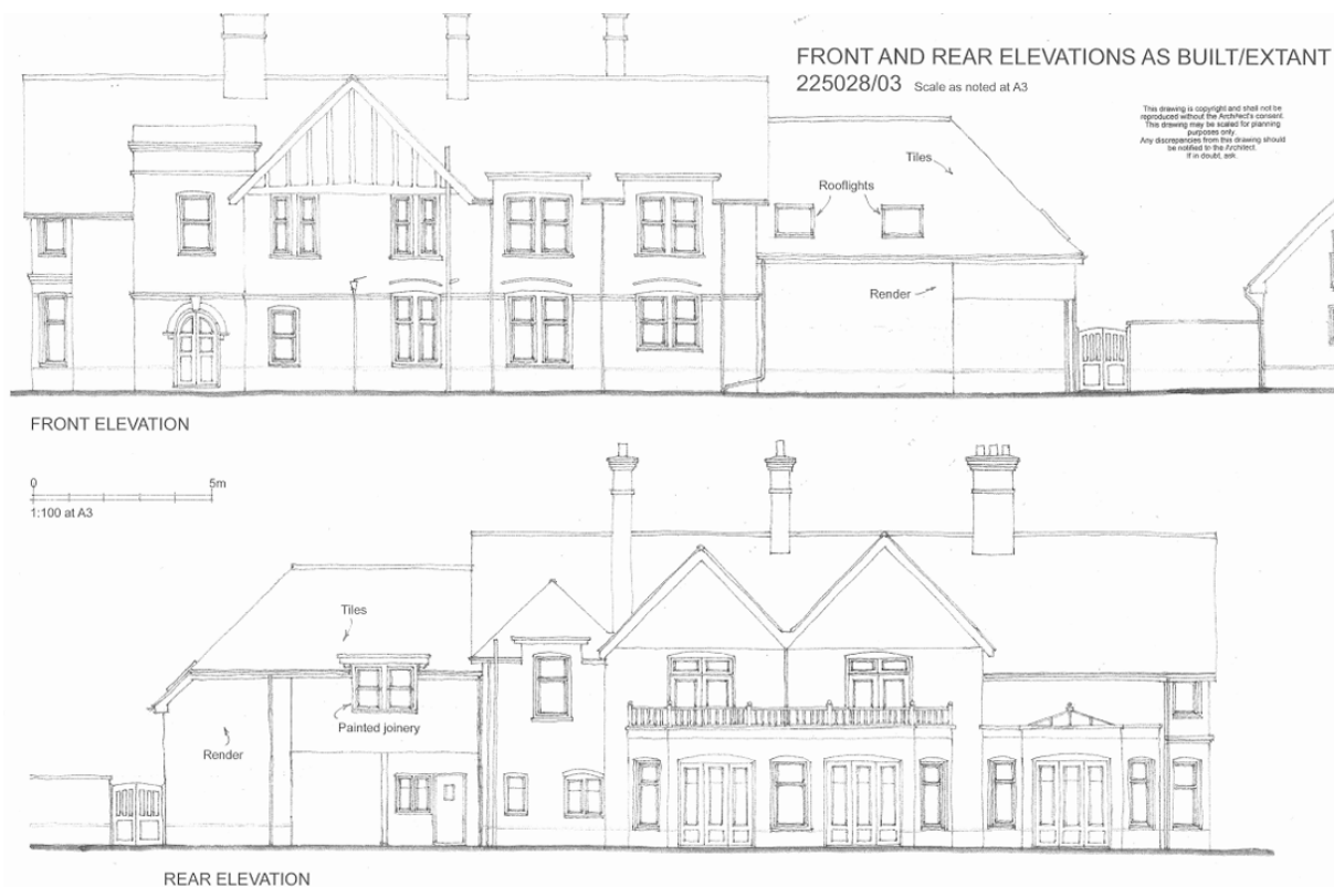
Figure 3 – Front and rear elevations as built out
