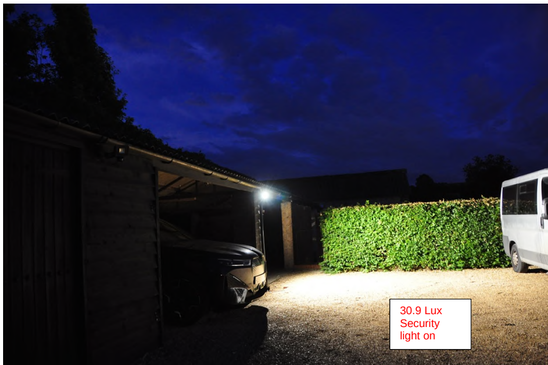
Plate 12 light spill from parking area light on short duration sensor
