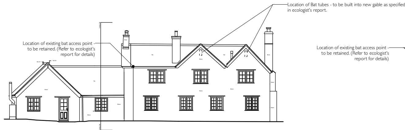
NORTH EAST ELEVATION (with new car port)
