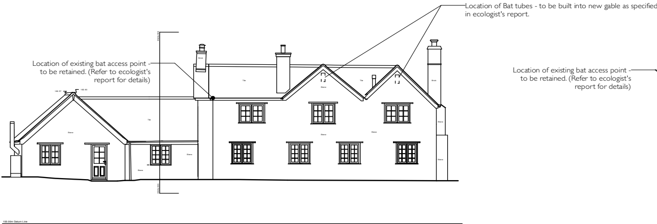
SOUTH WEST ELEVATION
