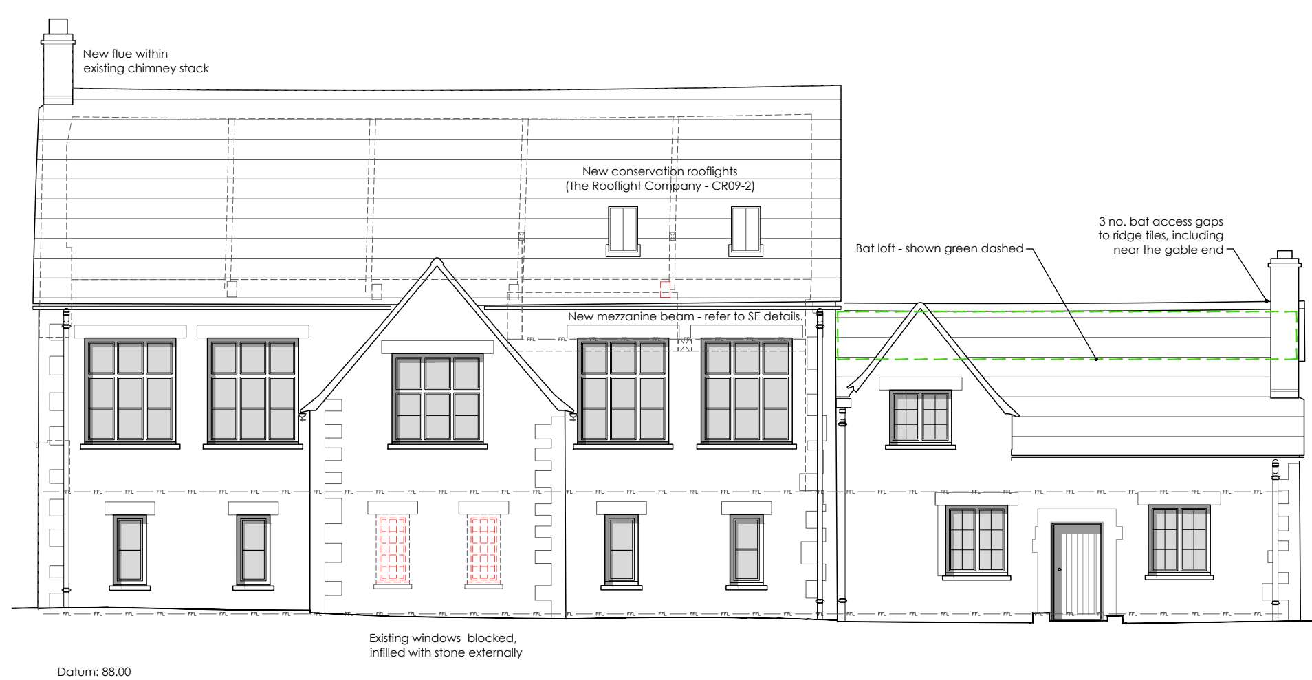
Courtyard / South West Elevation
