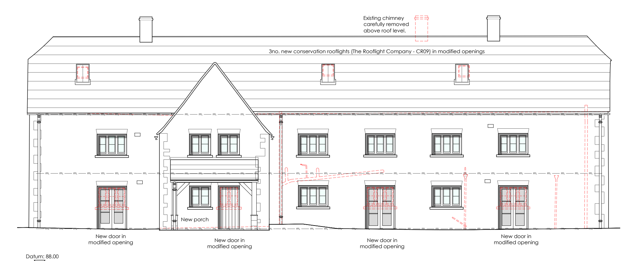
North West Elevation
