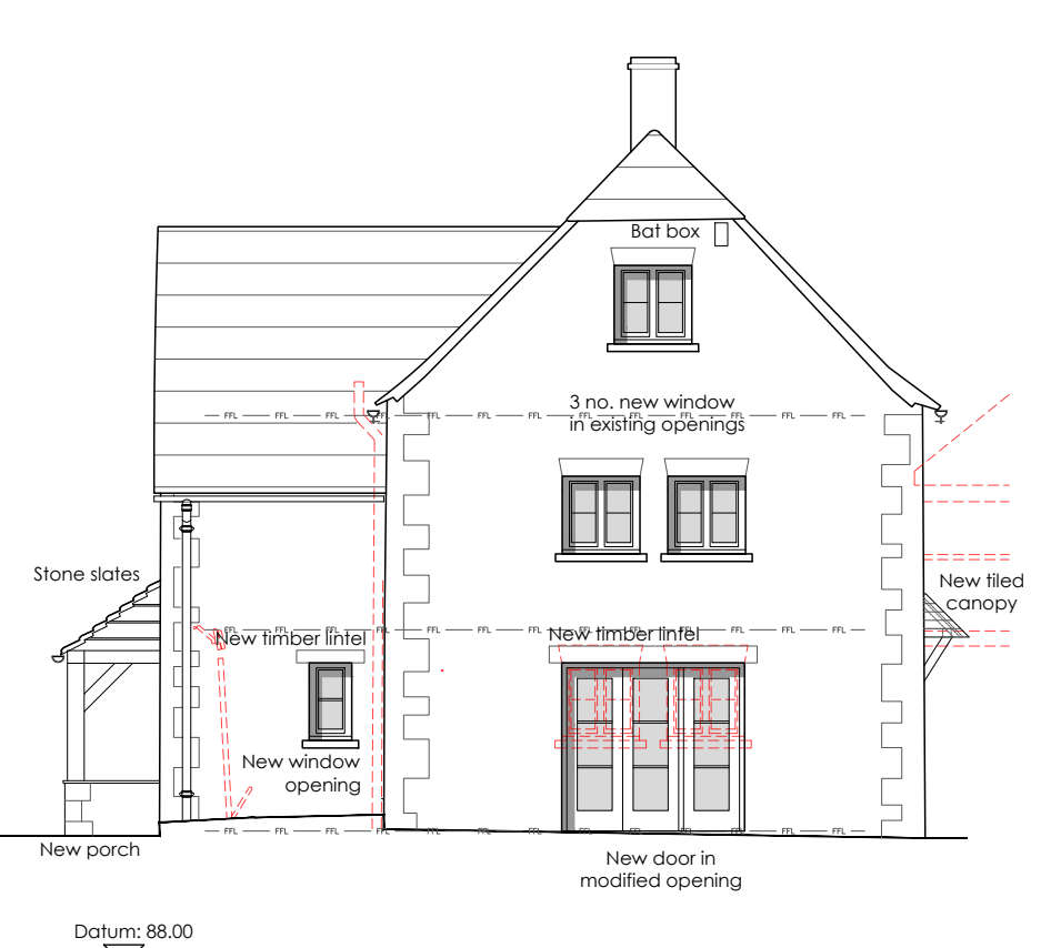
South West Elevation
