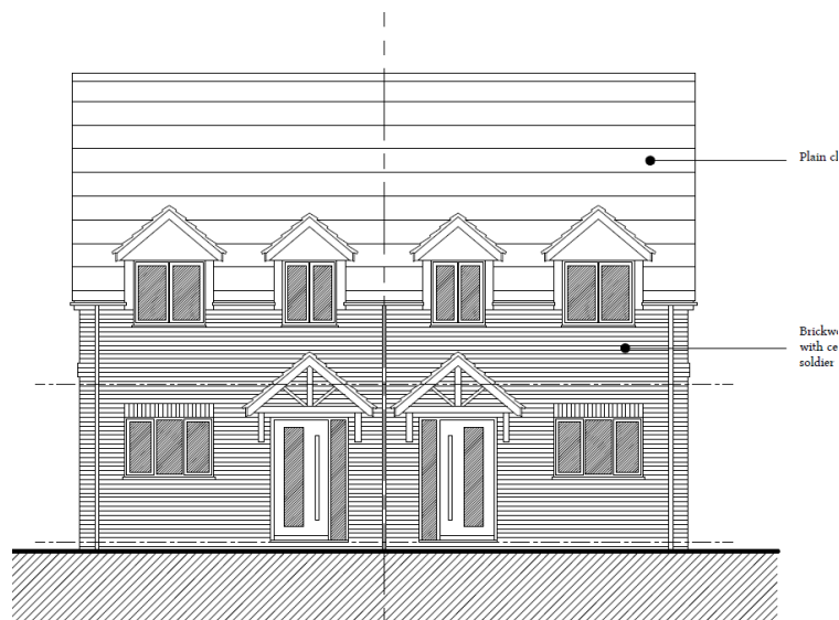
Figure 3: Proposed Elevation showing dormers in the roof
