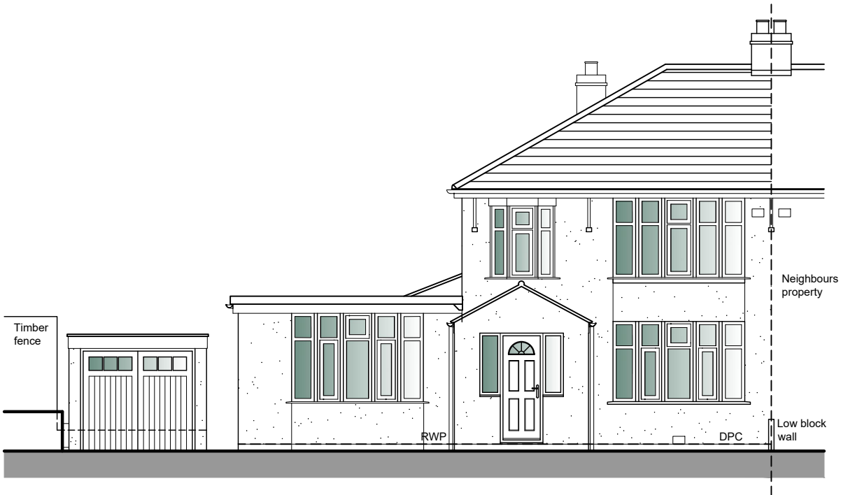
North West Elevation
