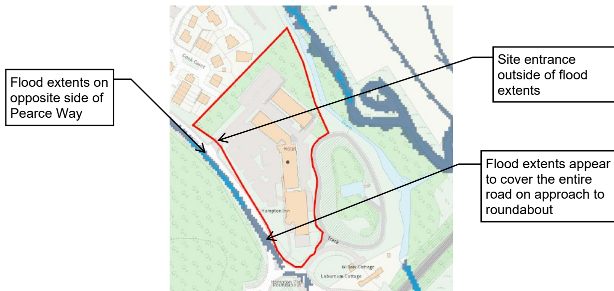
Figure 1: Surface water flood mapping showing the site entrance and flood extent on Pearce Way
