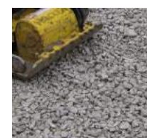
CGA type 4/20 (Clean stone) - permeable
