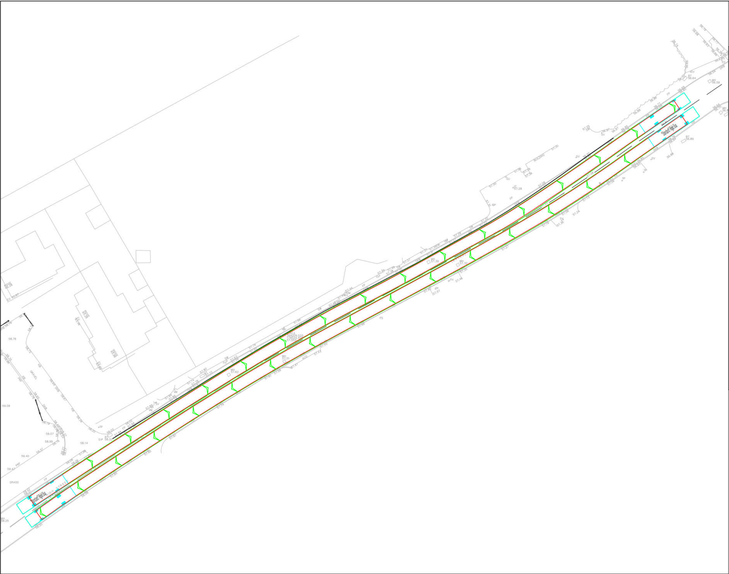
Swept Path Analysis of a Two 12m Buses Passing Each Other at Proposed Carriageway Narrowing
