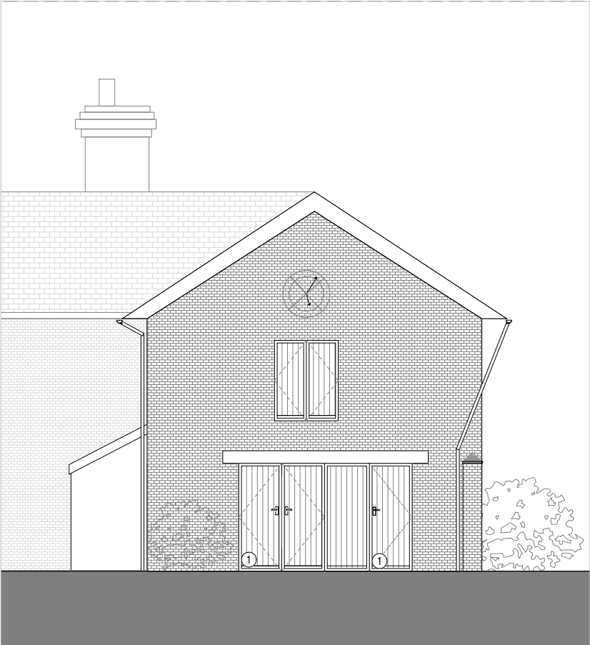
02- Proposed Front Elevation of barn (South)
