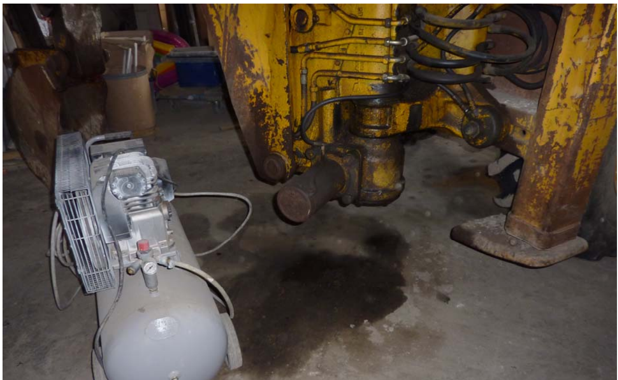
Figure 7: Staining on concrete floor beneath JCB in eastern building
