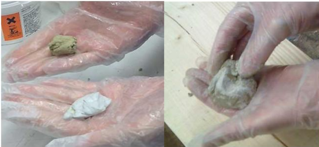
Priming wood with Epoxy Primer. Mixing Mouldable Epoxy
