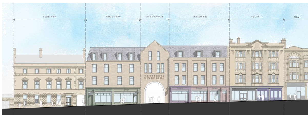
Figure 14: Extract from the Design and Access Statement detailing the proposed new High Street frontage over 3/4 storeys with existing 3-storey listed Lloyds Bank downhill and the 4-storey listed 22-23 up the hill.
