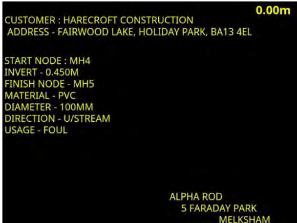
1, 00:00:00, 0.00 m Start node, manhole, reference: MH4
