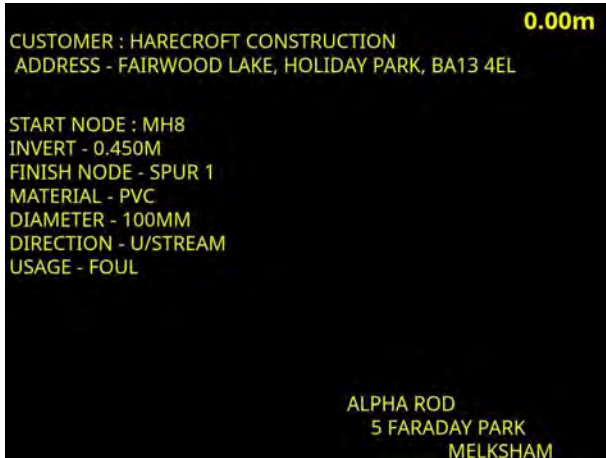
1, 00:00:00, 0.00 m Start node, manhole, reference: MH8
