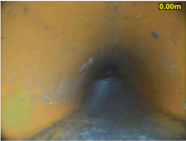
2, 00:00:15, 0.10 m Water level, 10% of the vertical dimension
