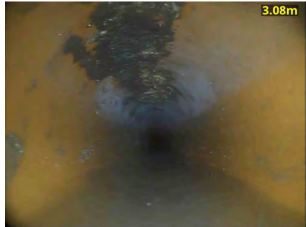
2, 00:00:29, 0.00 m Water level, 10% of the vertical dimension
