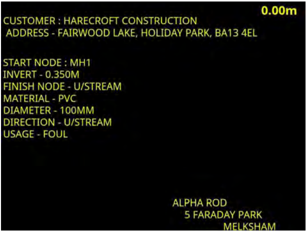
1, 00:00:00, 0.00 m Start node, manhole, reference: MH1
