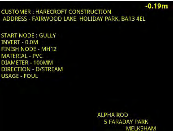
1, 00:00:00, 0.00 m Start node, gully, reference: Gully
