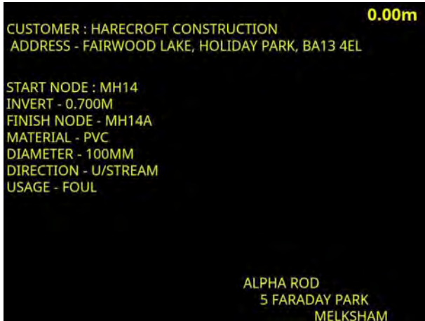
1, 00:00:00, 0.00 m Start node, manhole, reference: MH14
