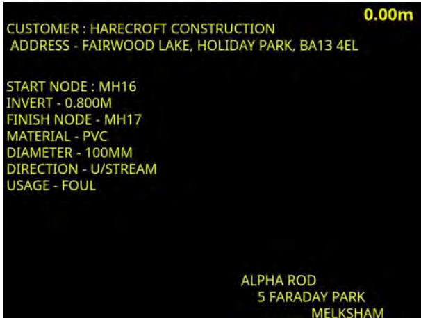
1, 00:00:00, 0.00 m Start node, manhole, reference: MH16
