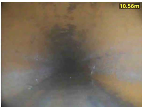
5, 00:01:20, 10.56 m Water level, 10% of the vertical dimension
