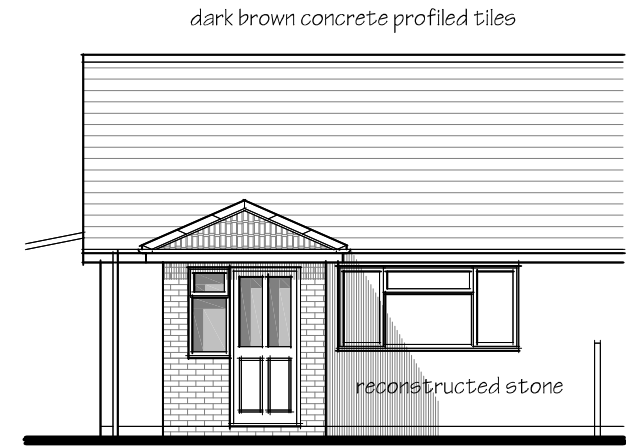
SOUTH WEST ELEVATION
