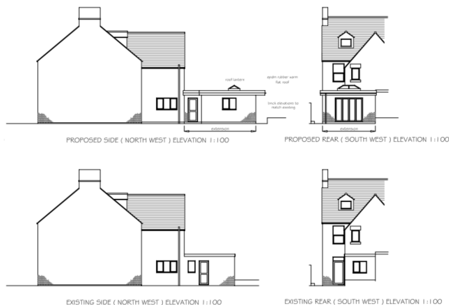
Figure 3: Existing and proposed side and rear elevations showing the scale and form of the replacement extension.
