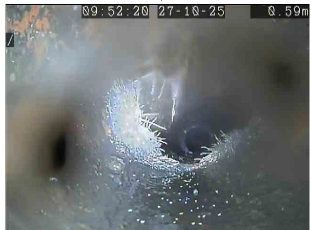
29b8a449-81a2-480e-afa3-6606c811843e.png, 00:00:37, 0.59 m Roots, mass, 5% cross-sectional area loss
