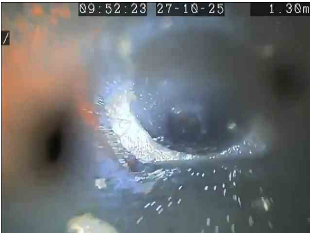
b6ac3f45-bb0a-4dc4-821e-189c033a0e48.png, 00:00:40, 1.30 m Joint displaced, medium
