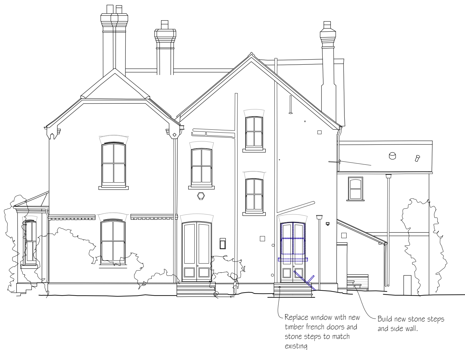
PROPOSED EAST ELEVATION 1:100
