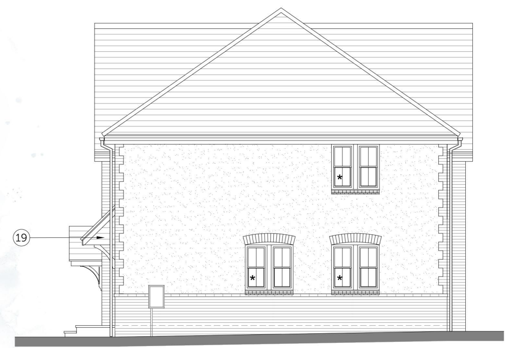
Side Elevation *Side window for plot 41 only
