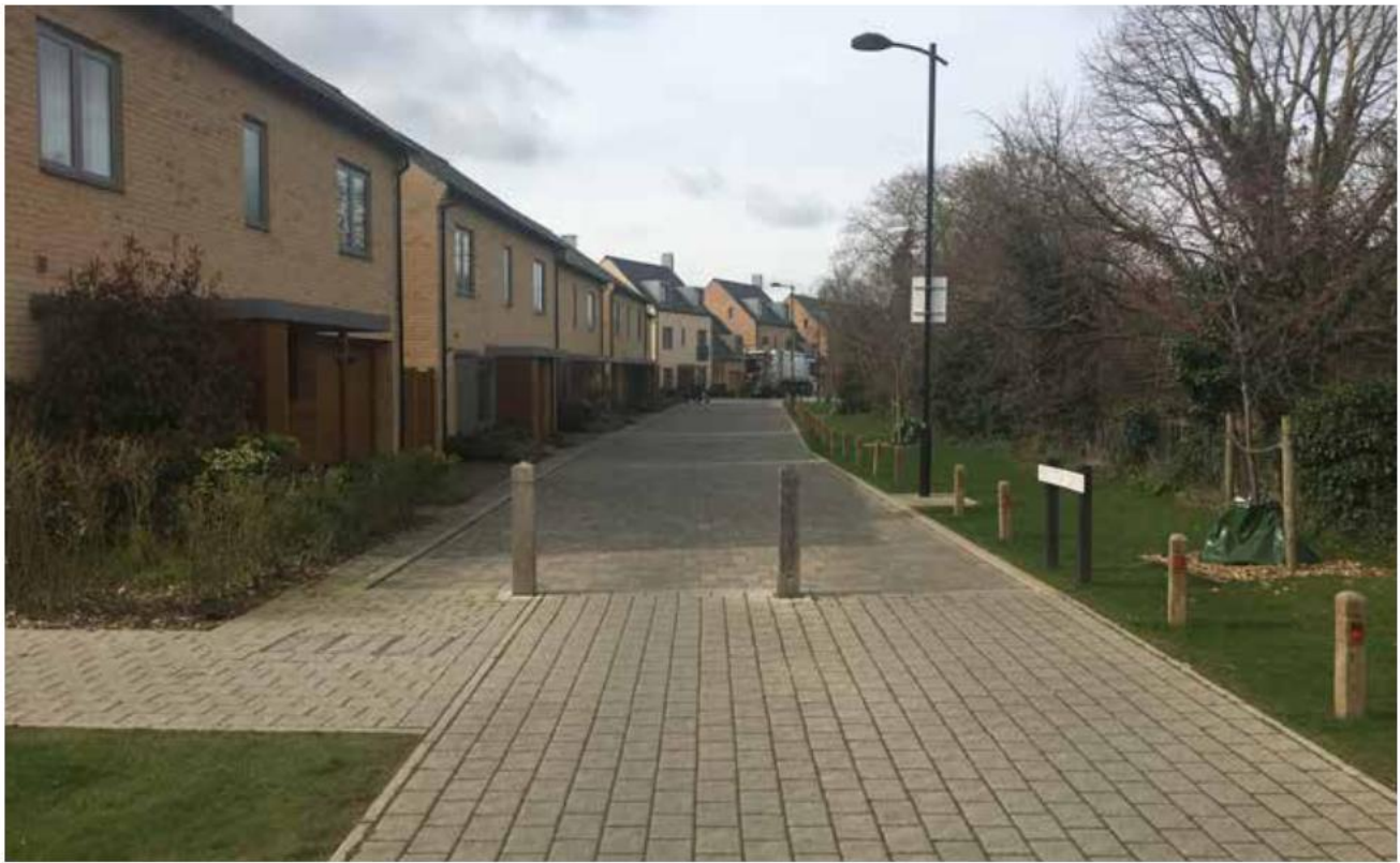
Edge lane example – Note the bollards to prevent vehicle passing by but allows people walking, wheeling and cycling to pass through without having to go around to another route.
