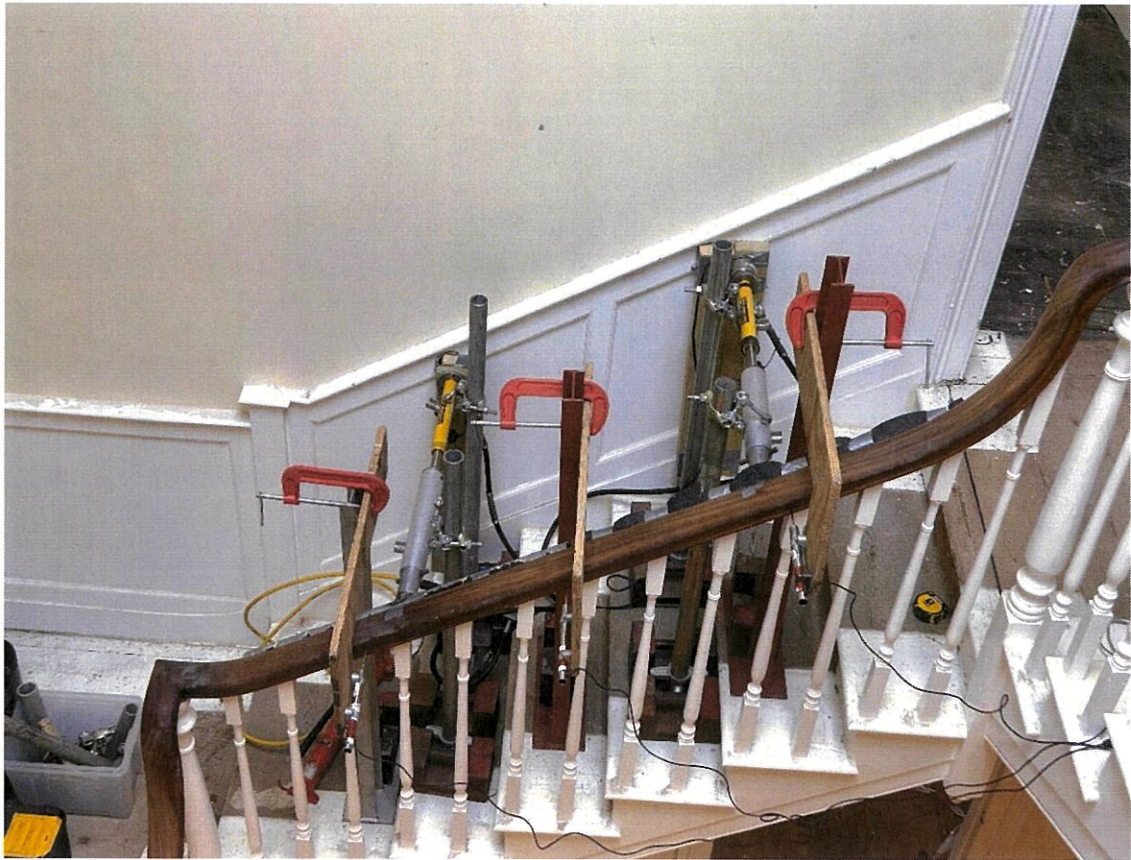
Photograph 3 Test setup for middle stair section
