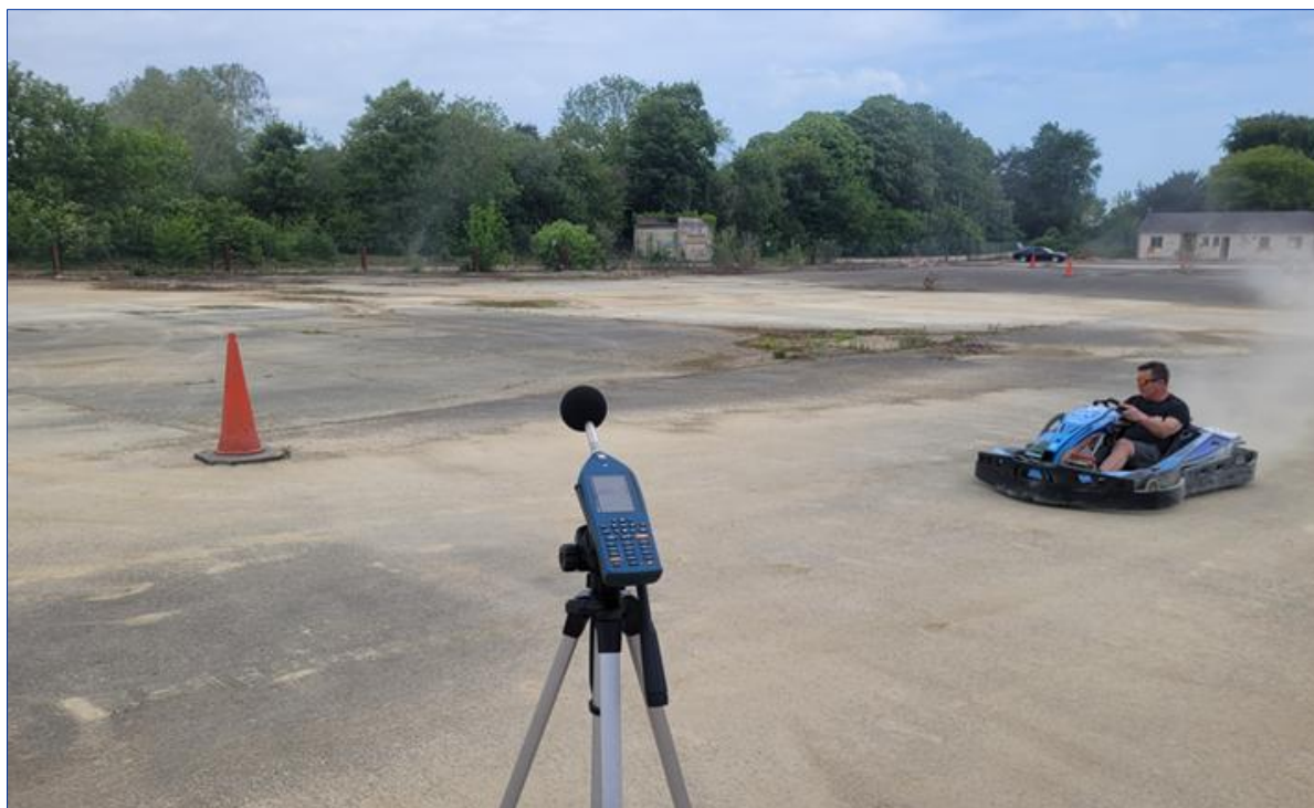
Figure 4.1: Measurement of Karting Noise
