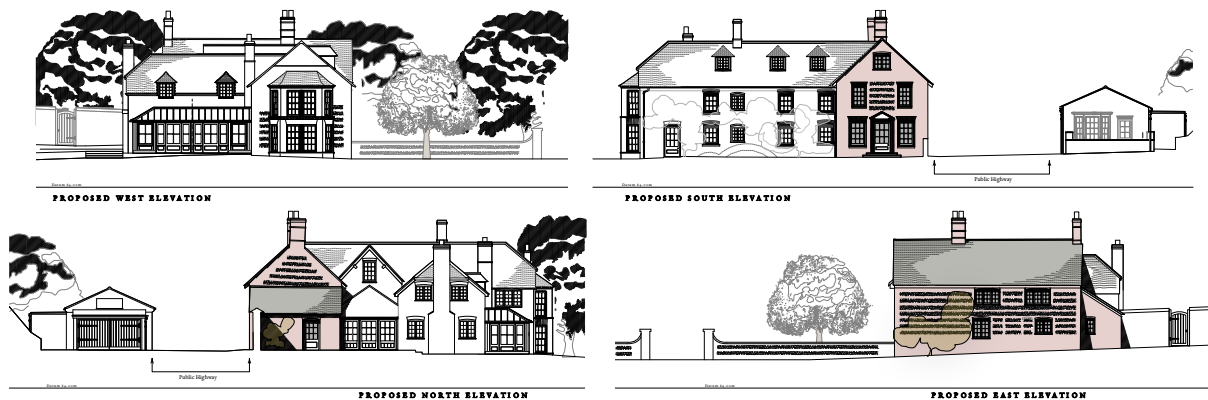
Above: Elevations highlighted to be carefully dismantled and reconstructed with the help of PER and cataloging materials.
