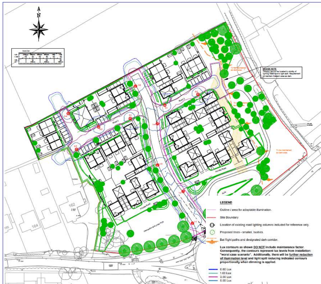
Figure 10: Extract of the lighting plan and lux contours for the proposed development
