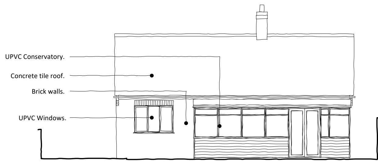
1:100 - Existing North Elevation
