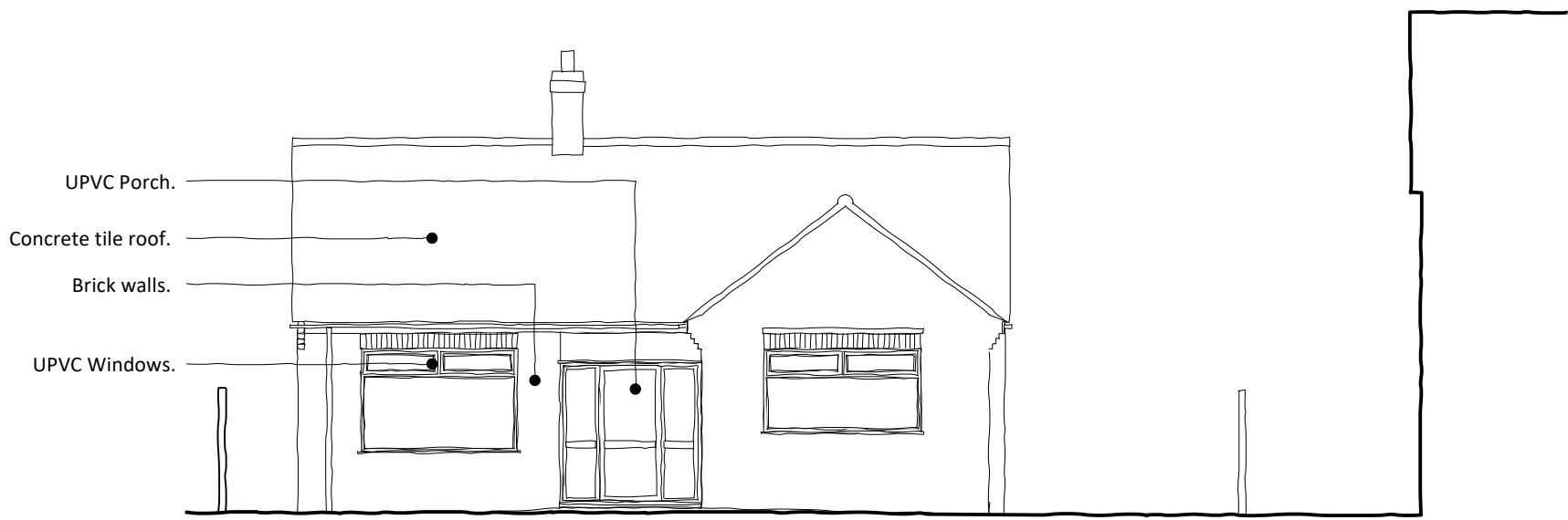
1:100 - Existing South Elevation
