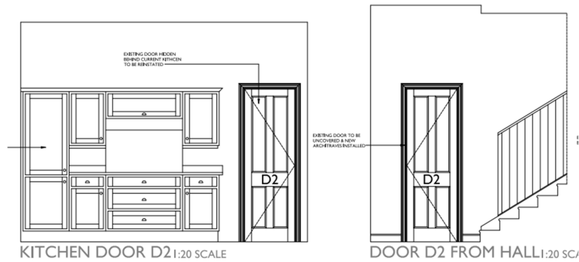
Fig.5 Reinstatement of Original Door to Back Stairs.
