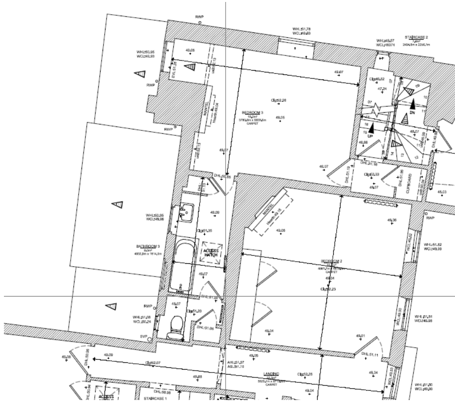
Existing first floor plan
