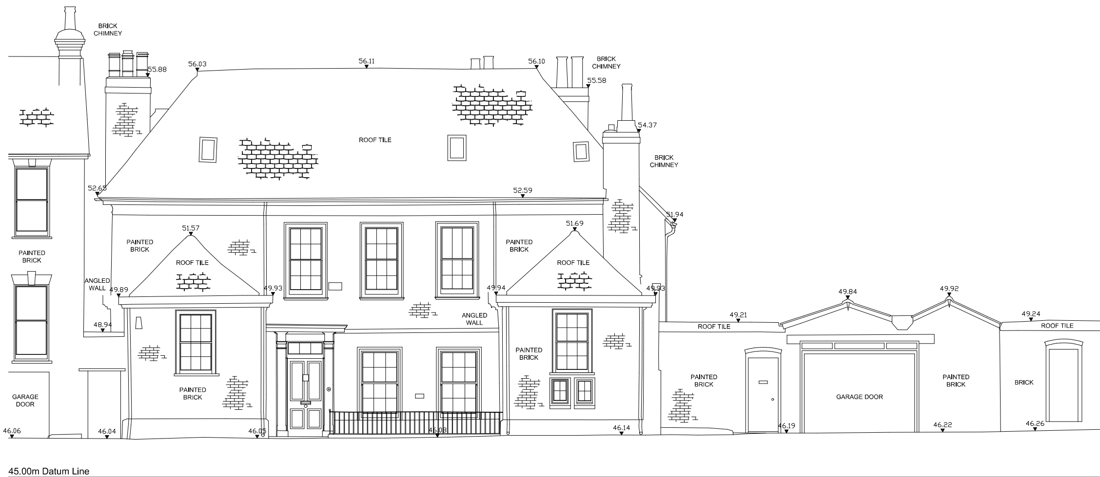
45.00m Datum Line EAST ELEVATION
