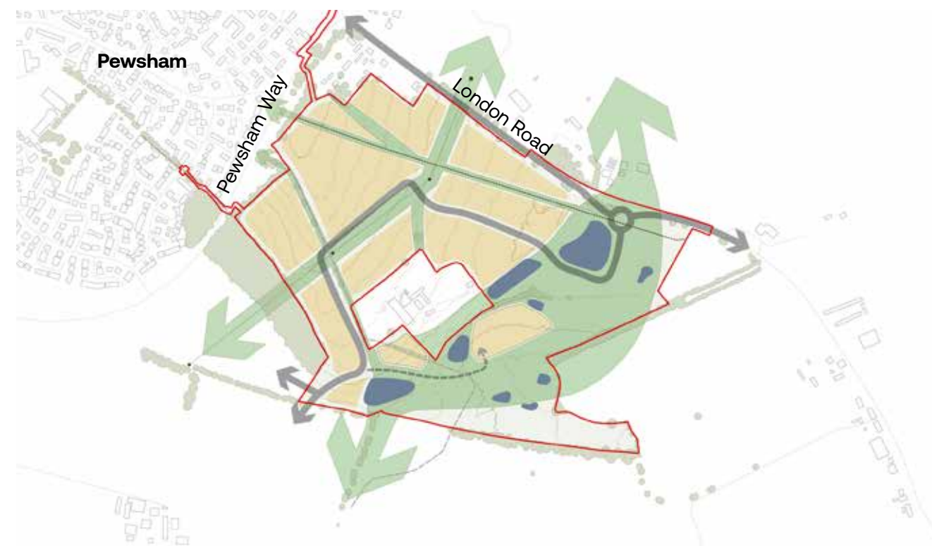
Figure 6.4 Attenuation basins positioned in areas of flatter topography.
