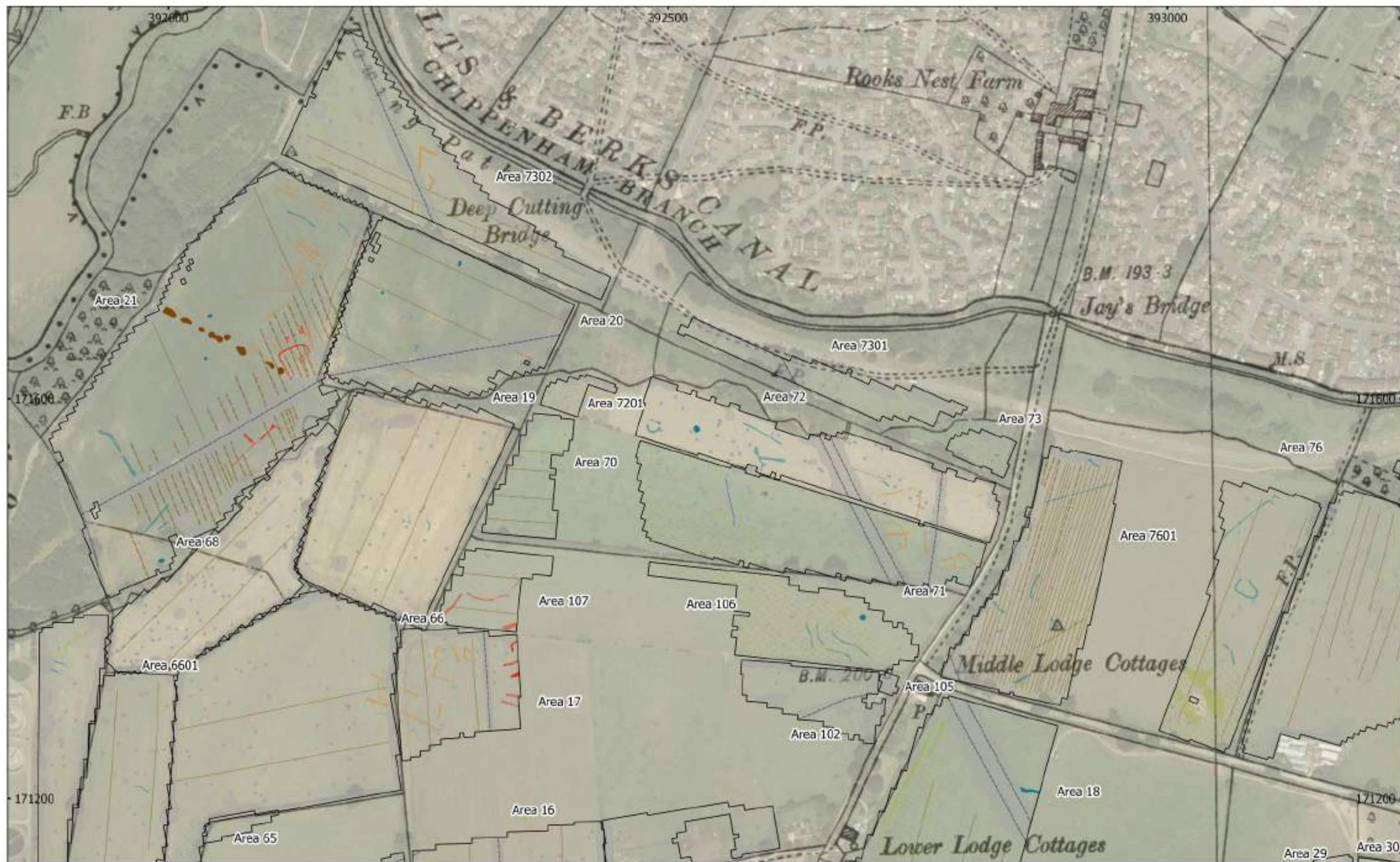
MSST1037 - Chippenham Development Figure 4 - Magnetic Interpretation Over Historical Maps and Satellite Imagery (Overview) (Northern Areas) 1:3,500 @ A3 Copyright Magnitude Surveys Ltd 2022 Contains historical mapping © CLS Data 2022: Ordnance Survey, 6" 2nd edition c. 1882-1913 Contains satellite imagery © 2021 Bing Satellite
