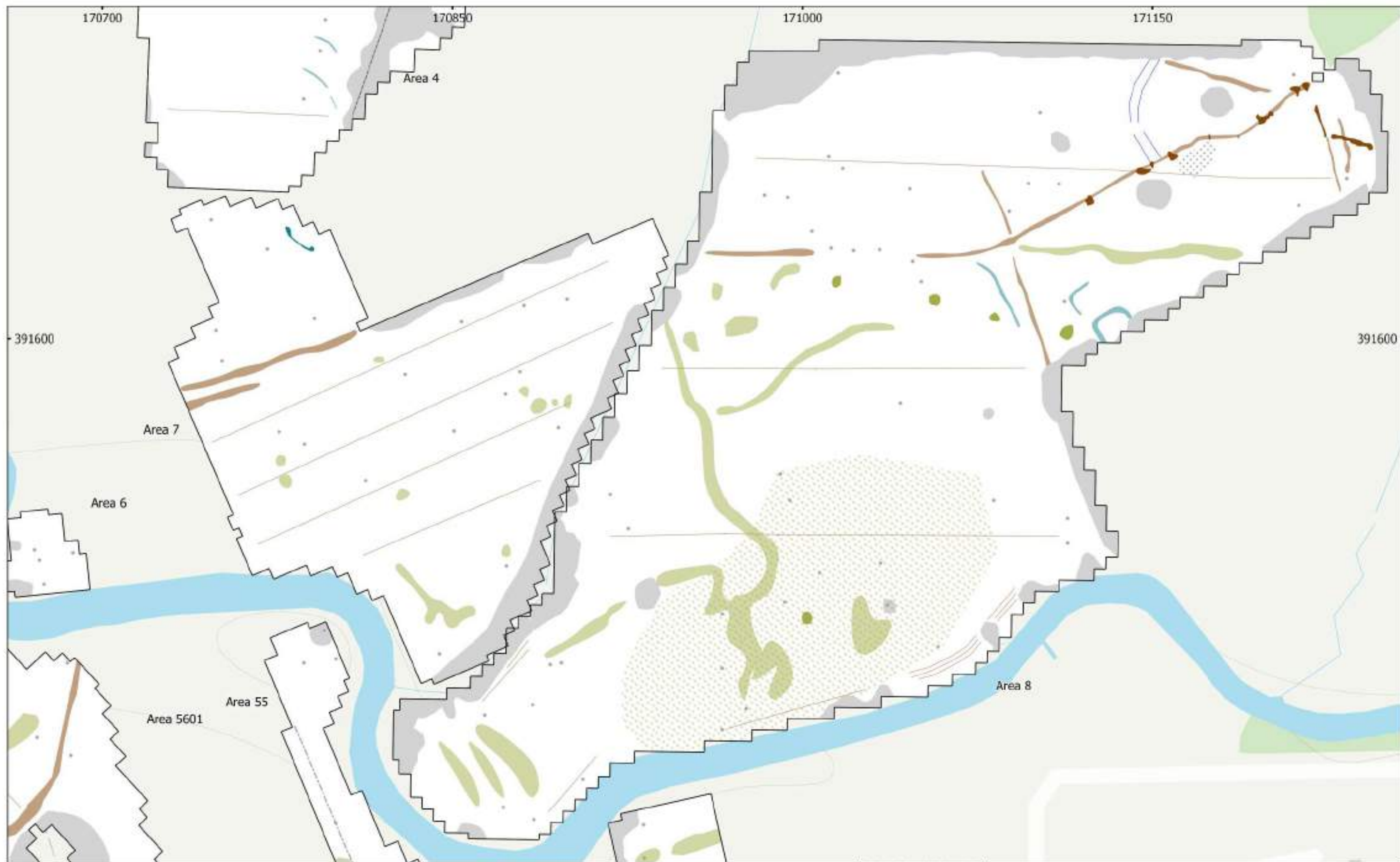
MSST1037 - Chippenham Development Figure 35 - Magnetic Interpretation (Areas 4, 6, 7, 8 and 5601) 1:1,500 @ A3 Copyright Magnitude Surveys Ltd 2022 Contains Ordnance Survey data © Crown Copyright and database right 2022
