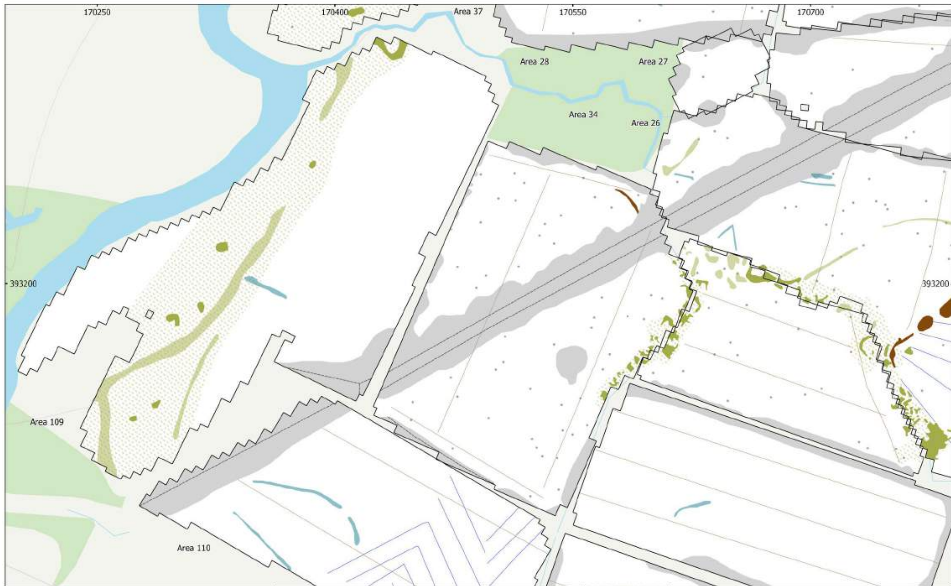
MSST1037 - Chippenham Development Figure 62 - Magnetic Interpretation (Areas 23, 24, 26, 27, 28, 33, 34 and 37) 1:1,500 @ A3 Copyright Magnitude Surveys Ltd 2022 Contains Ordnance Survey data © Crown Copyright and database right 2022
