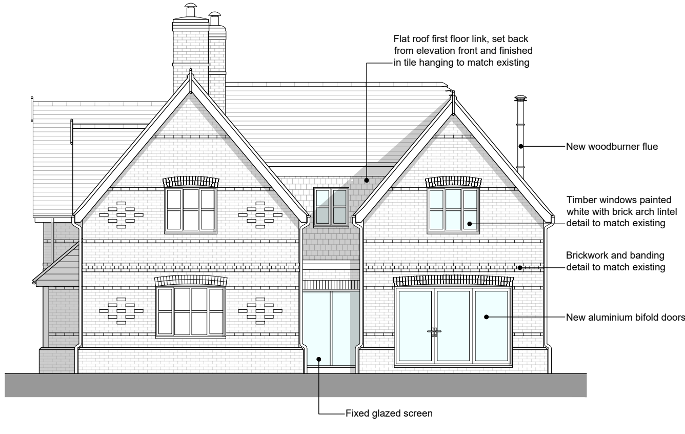
PROPOSED NORTH ELEVATION Scale 1:100
