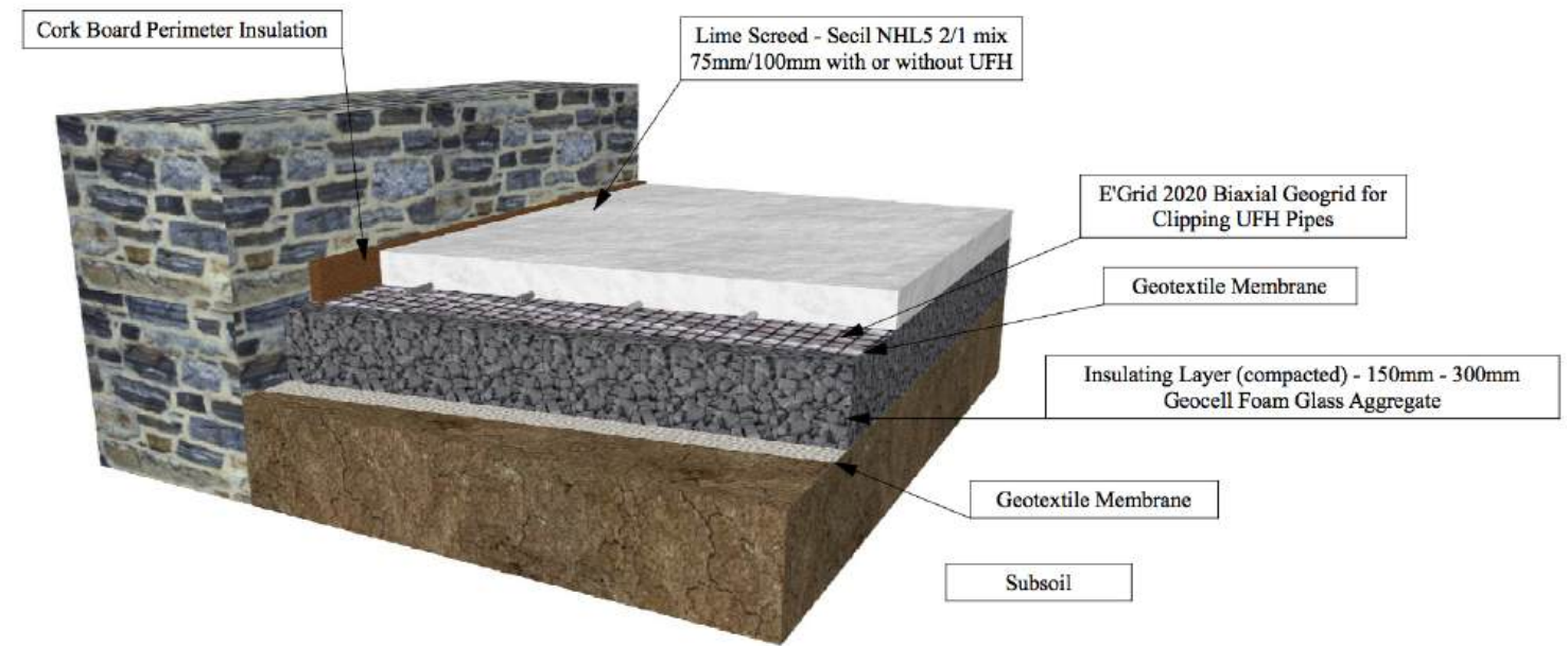
Mike Wye - Limecrete and Geocell foam glass and replacement ground floor construction for R001 / R006 / R007
