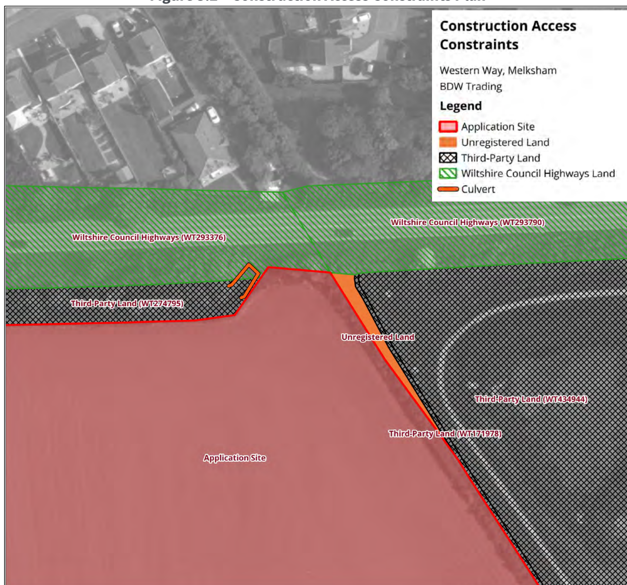
Figure 3.2 – Construction Access Constraints Plan
