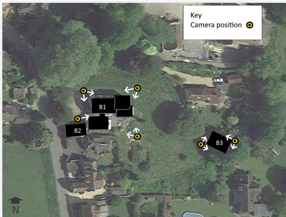
Figure 4. Map illustrating the location and number of surveyors and/or infrared cameras to robustly assess the buildings
