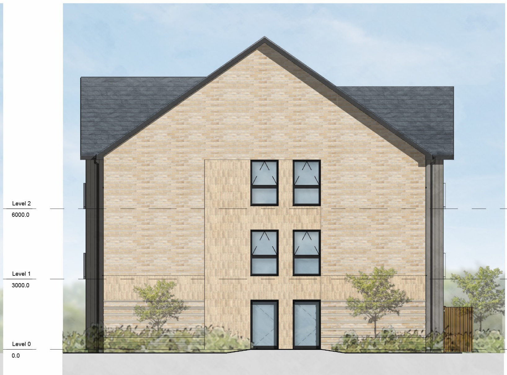
5 Gable Elevation - East Wing 1 : 100
