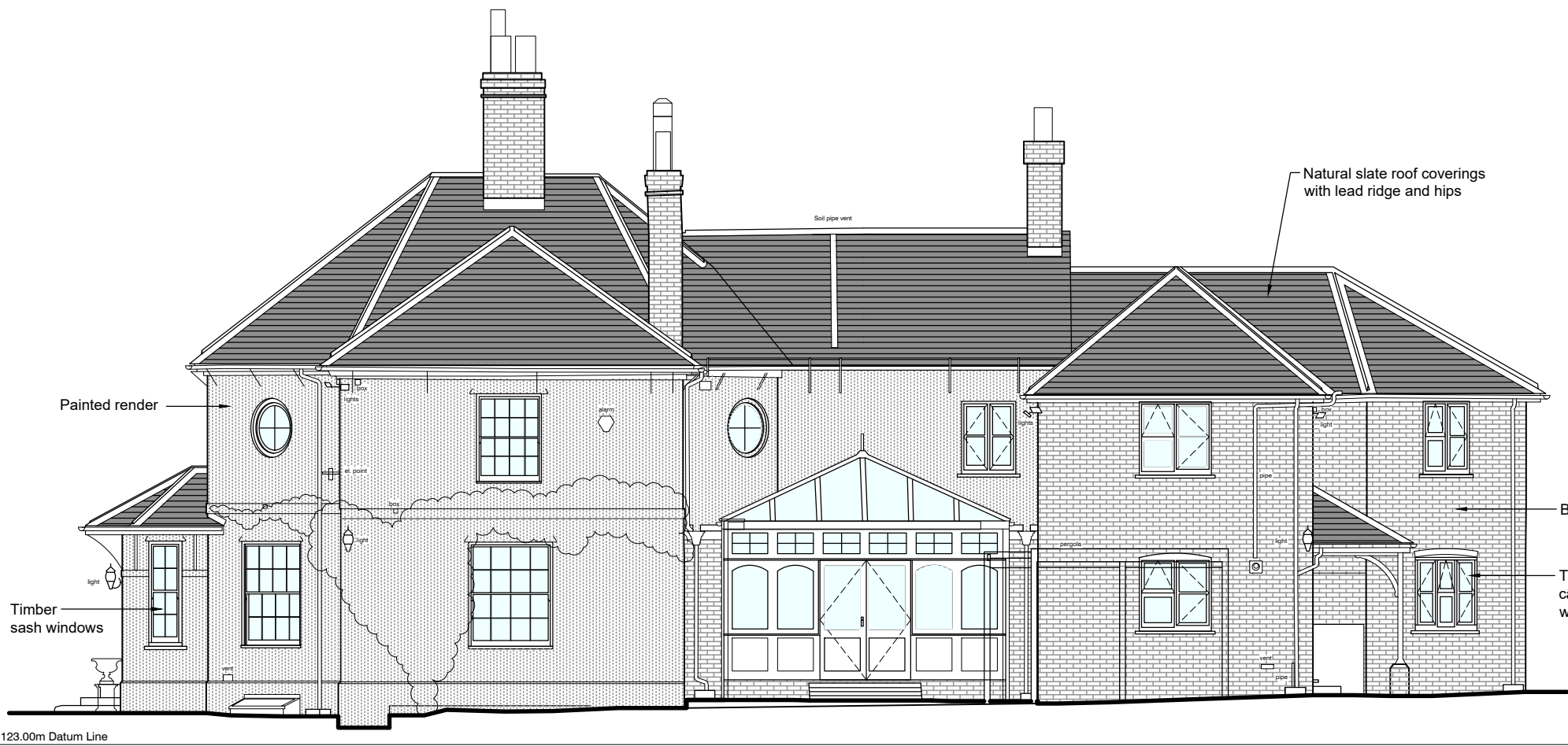
EXISTING FRONT ELEVATION (north-east) Scale 1:100
