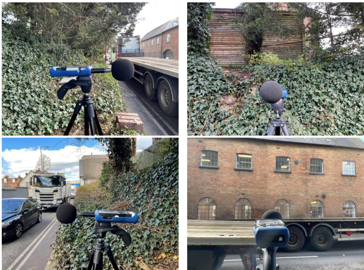
Figure A.4.1 - Spot Measurement S1 in situ
