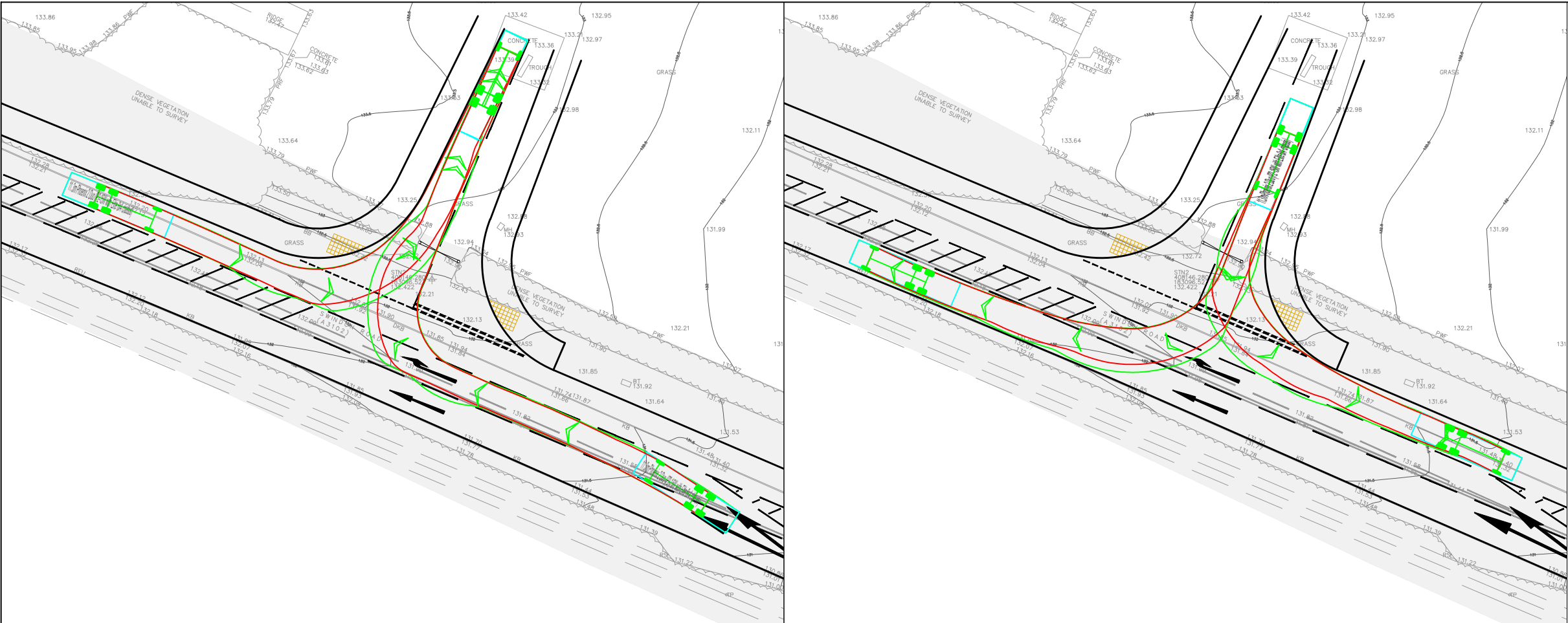
Swept Path Analysis of an 11.3m Refuse Vehicle Entering and Egressing Access
