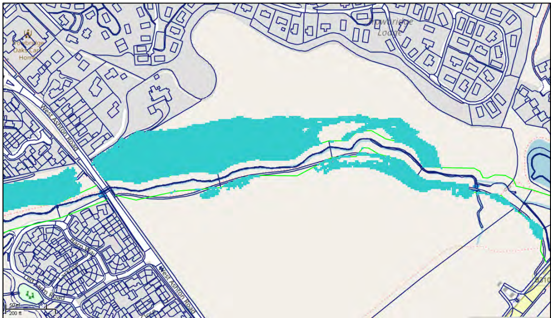
Figure 5.3: Extent of flooding from Blackball Brook for the 1:1000-year event
