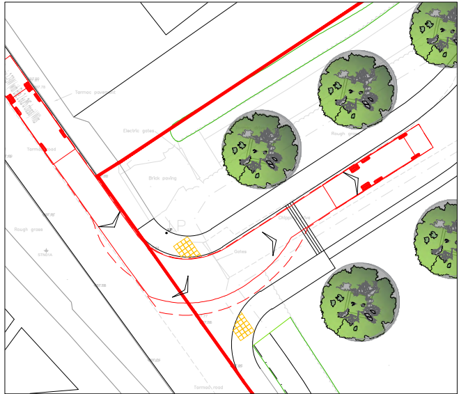
Inset 1: Refuse vehicle entering site
