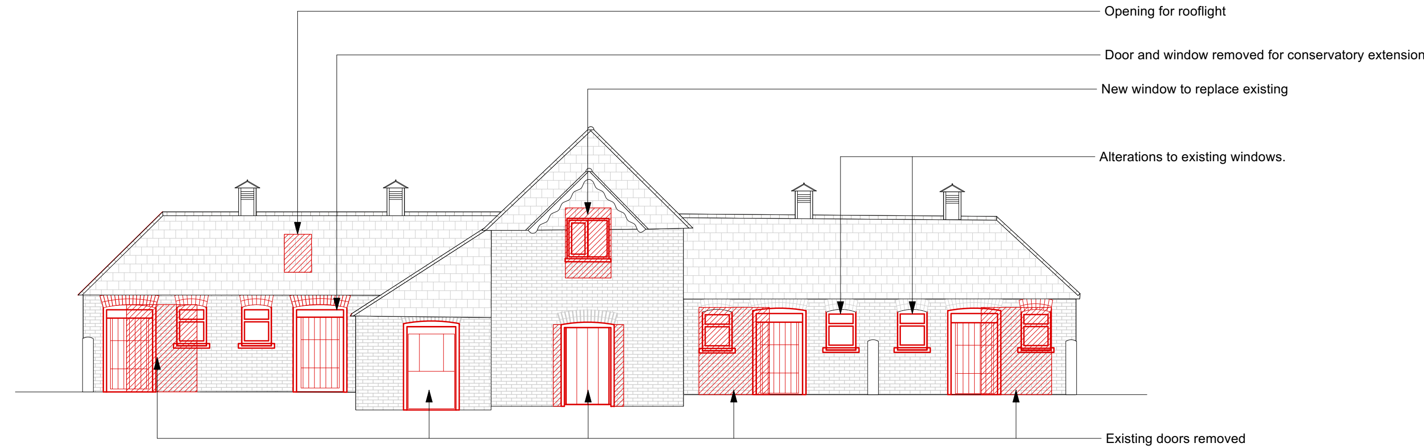
Existing Southerly Elevation Proposed Demolition Scale: 1:100
