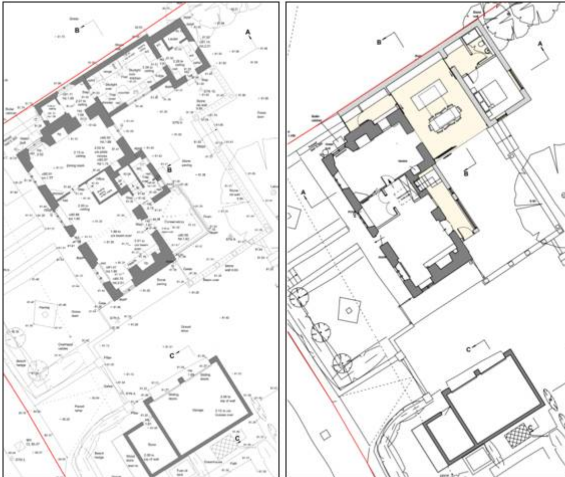
Existing and Proposed Ground Floor Plans – increased rear projection of 3.3m, same width, and approx. 0.7m floating roof infill to rear boundary
