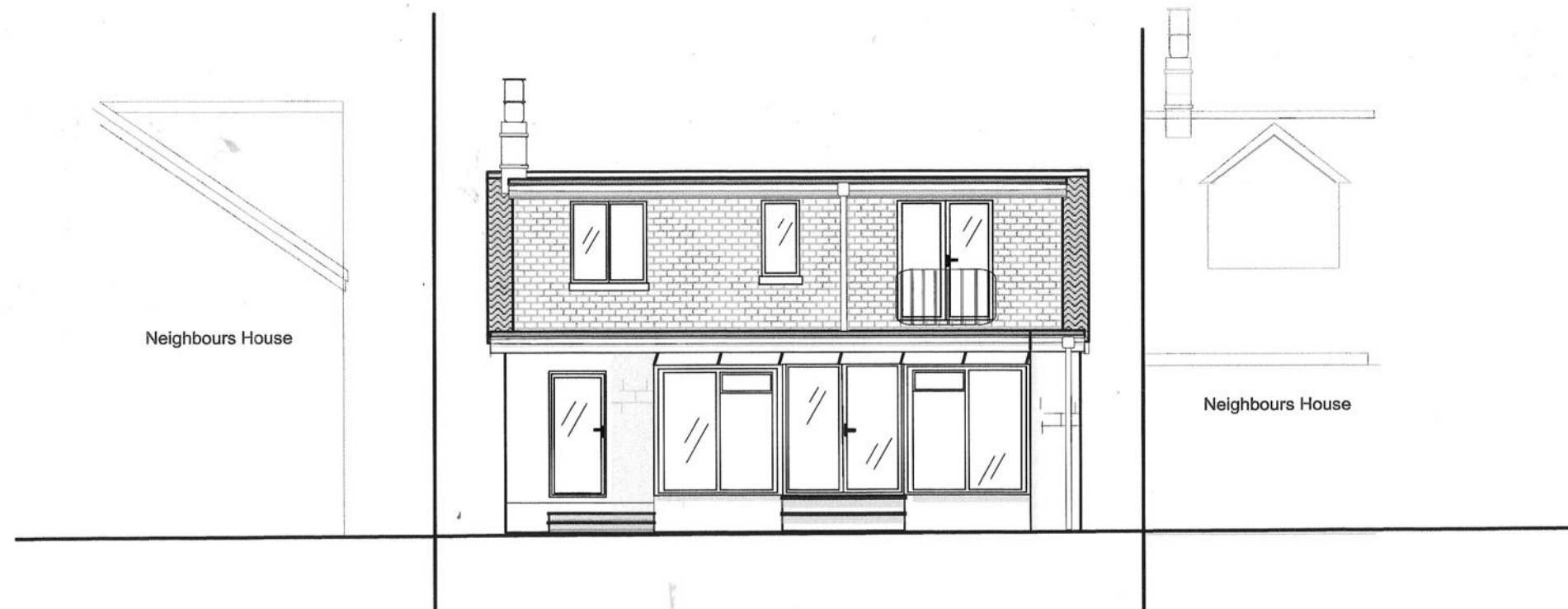
Existing Back Elevation
