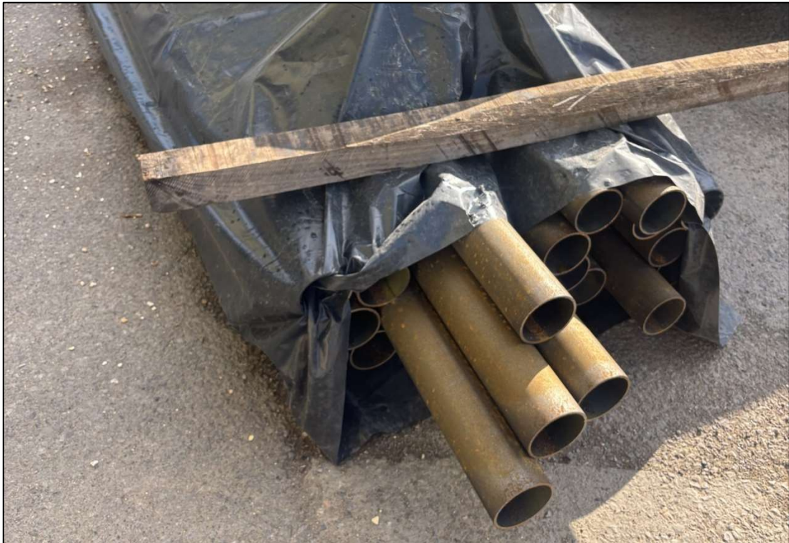
Image 1: Existing untreated steel stored externally beneath temporary tarpaulins. Exposed parts rusting
