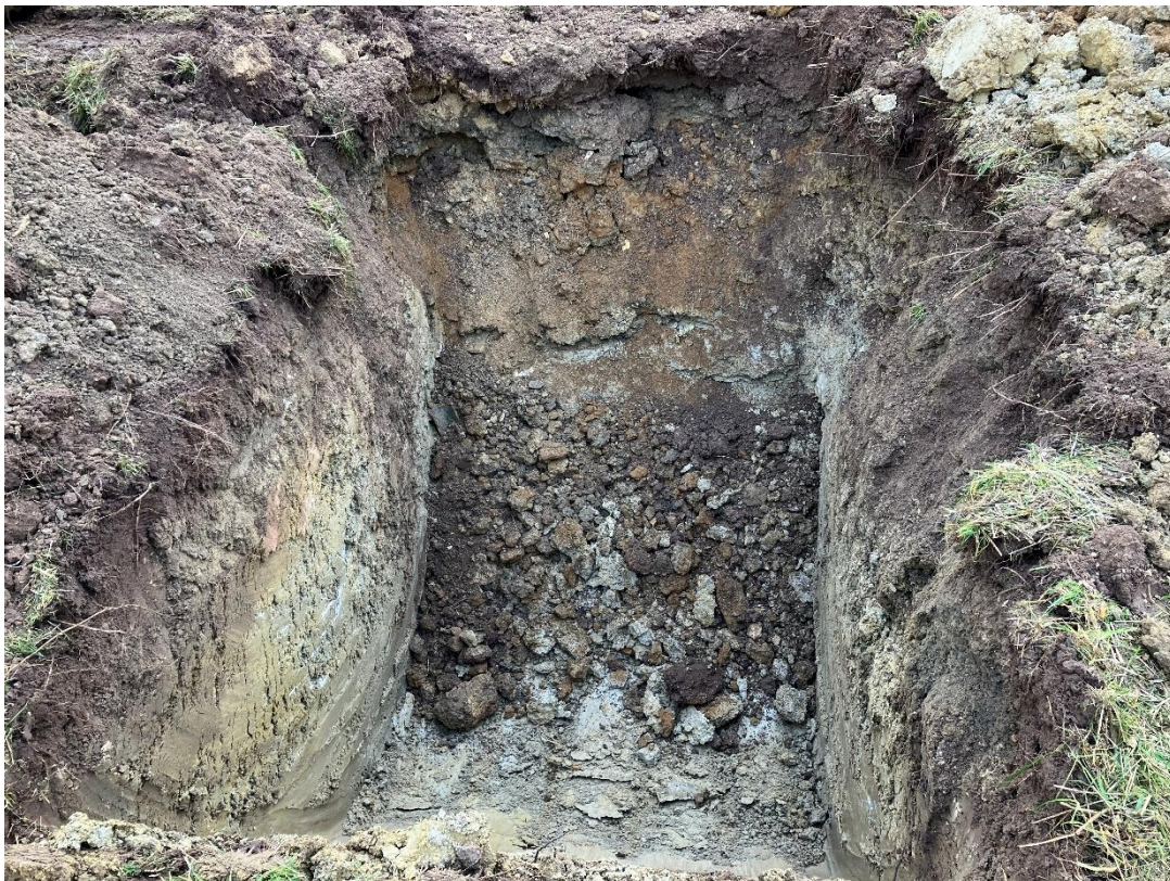
Photograph 12 – Side view of TP312 and its arisings, excavated to 1.90m bgl.
