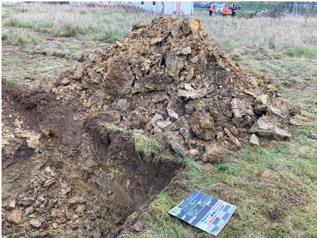
Photograph 10 – Side view of TP310 and its arisings, excavated to 1.51m bgl.
