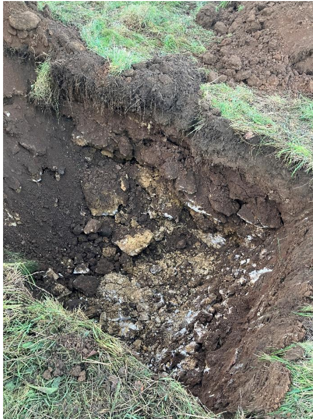
Photograph 15 – Side view of TP316 and its arisings, excavated to 1.60m bgl.
