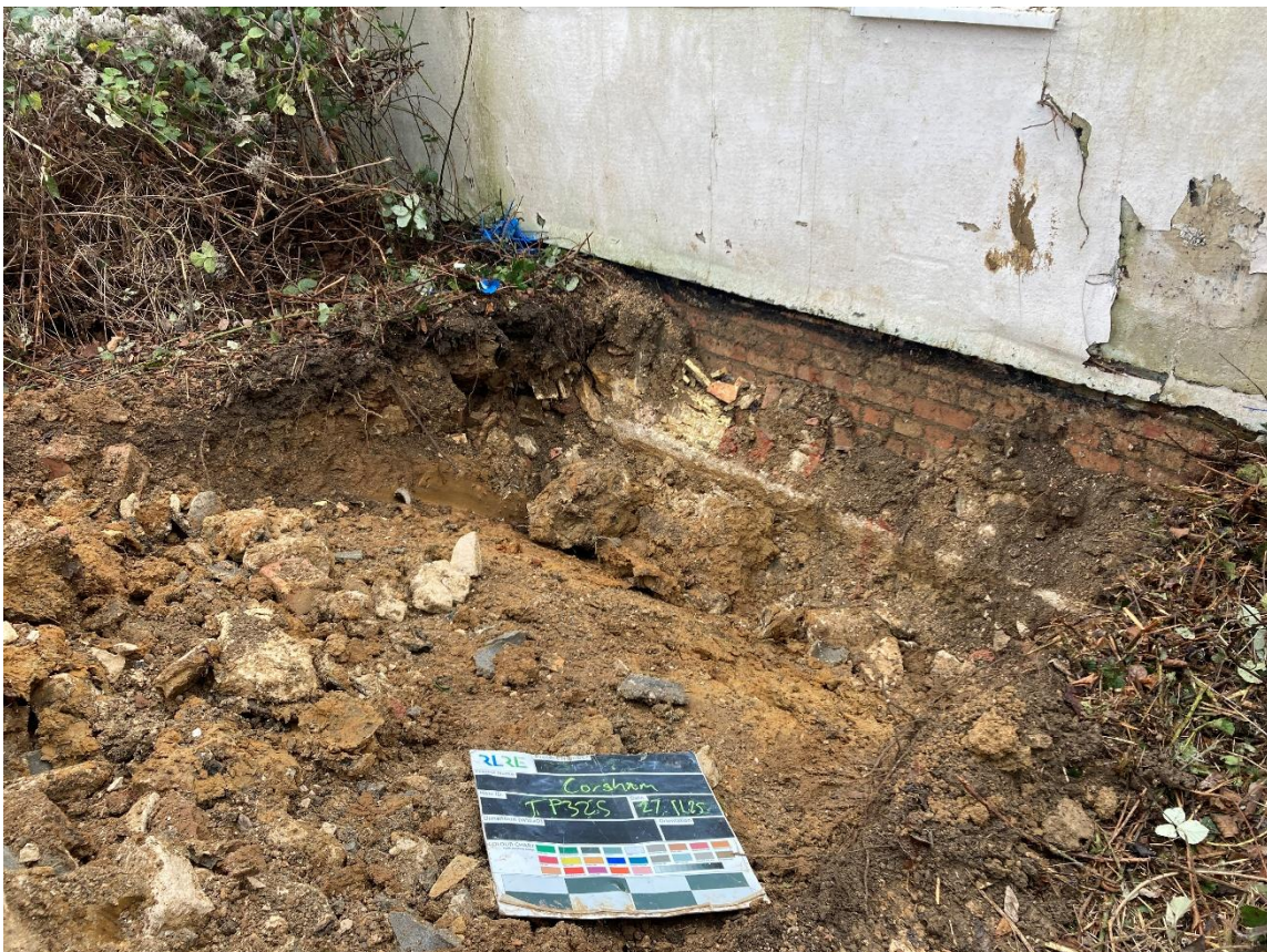
Photograph 20 – Side view of TP325 and its arisings, excavated to 0.94m bgl.
