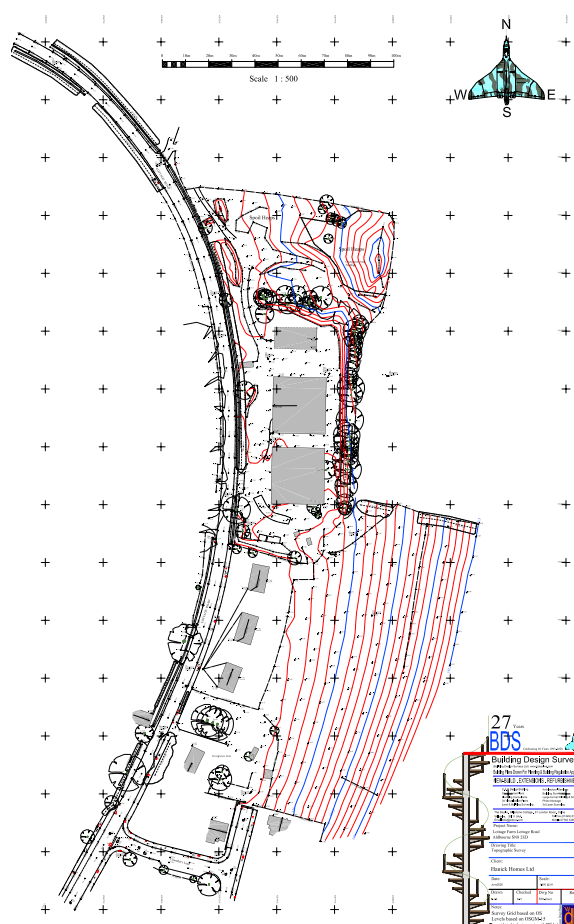
Existing site topo showing contours
